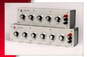
Guildline Model 9340 Series of Precision Decade Resistance Boxes is a complete family of easy to use resistance standards offering the best combination of highest accuracy and widest range commercially available. There are 5 standard types available from 3 dial to 7 dial. The smallest increment offered is  $10m\ \Omega$  and the largest full scale total resistance available is just over  $10T\ \Omega$ . All full scale resistance values in the range are available in all the dial sizes.
